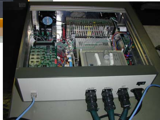
control unit of calibration lamp source
