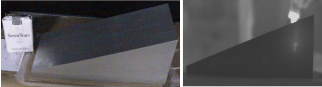
Fig. 8 Visible (left) and infrared (right) photographs of germanium prism. (120 x 120 x 270 [mm]) Heated solder could see through a germanium of 120 mm in thickness by means of infrared camera.
