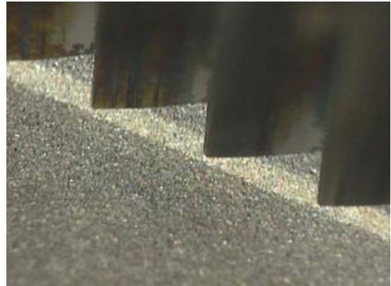
Fig. 5 Prototype germanium immersion grating (30 x 30 x 72 [mm],  $a = 68.75$  [deg.], 1.67 [grooves/mm]).
