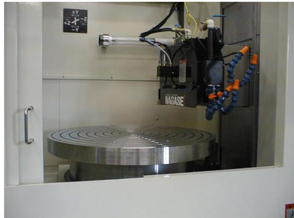
Fig. 16 Rotary grinding/turning machine with turntable of 800mm in diameter and 10 nm accuracy in control resolution.
