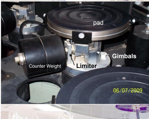
Axial Support System: a mirror-touching pad, its counter weight, gimbals, and its limiter
